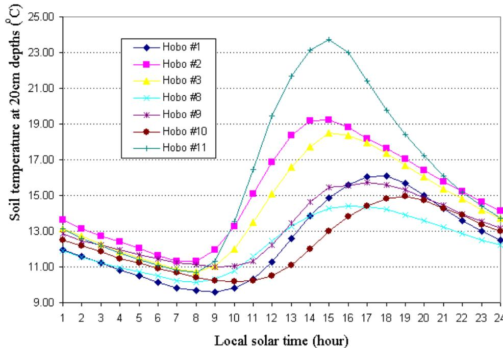
Fig. 2. Diurnal patterns of soil temperature for different spatial location during late summer (10-Aug-98 to 9-Sep-98, measurements averaged for each time hourly interval).
