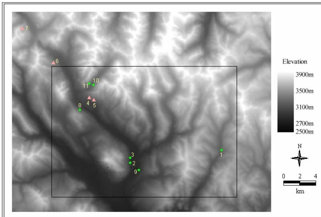
Fig. 1. Locations of soil temperature sensors shown on the DEM for the immediate vicinity of RMBL. Circles indicate sensors used in this analysis ( $n=7$ ) and triangles indicate sensors that did not collect usable data during the first year of study ( $n=4$ ).
