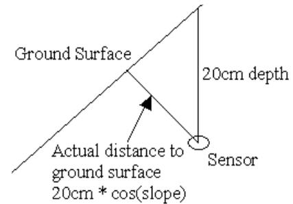
Fig. 4 Actual distance between sensor and ground surface on a slope.
